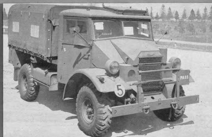
GENERAL SERVICE TRUCKS —Are quickly adaptable for transport of men and supplies, as the need may arise. Mobile work shops are mounted on this type of truck for quick repairs in the field.
